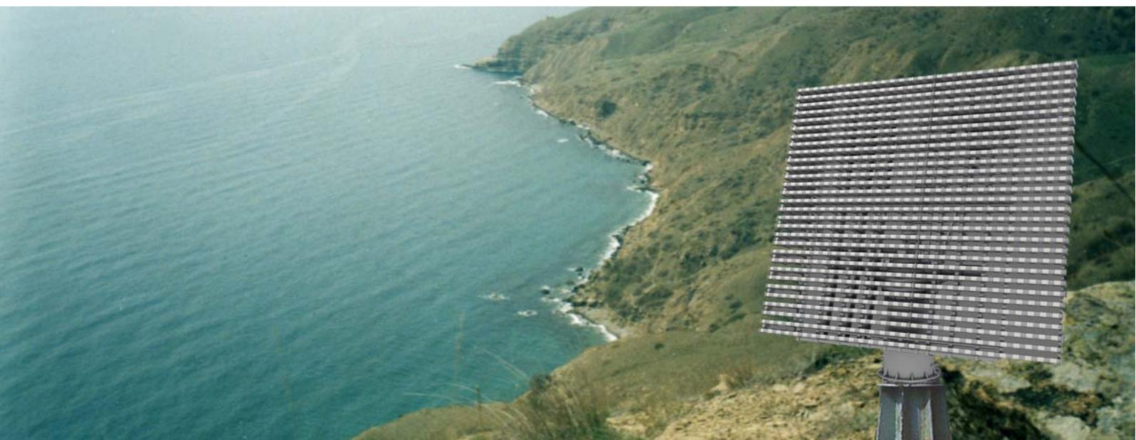
“Podberezovik-ET1” radar is intended for aerial and surface targets detection and designation for fire means. The radars are deployed both on medium and large displacement warships and coastal warning stations.
